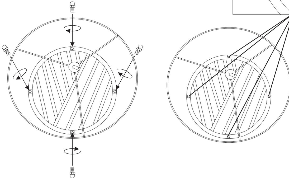
**Step 3:** Now, Tighten screws (C) on all 4 sides in clockwise direction by using wrench (D).
