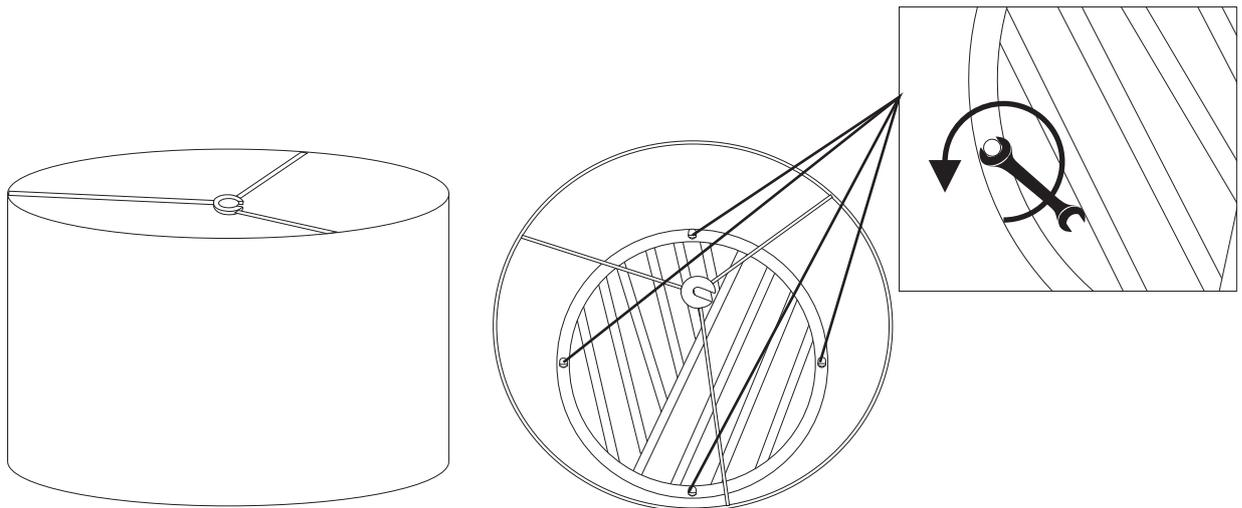
**Step 1:** Unscrew all 4 Screws (C) from old shade (A) in anti-clockwise direction using wrench (D).
